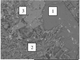
TM3030\_0585 2024.03.28 14:40 N D7,9 x100 1 mm Straw before biodegradation
