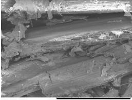
TM3030\_0573 2024.03.28 14:08 N D8,3 x100 1 mm Straw after biodegradation
