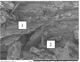
TM3030\_0575 2024.03.28 14:12 N D8,0 x100 1 mm Straw after biodegradation
