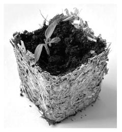
Fig. 4. Finished product – seedling pot. A rough surface of the walls can be observed under the influence of moisture and visible light, the straw-carrageenan composite easily
