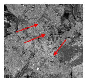
Fig. 3. SEM image – straw glued with carrageenan before degradation. The contact angle of the composite joint in the arrowed locations is close to 0, magnification 400x, tabletop microscope HITACHI TM3030
